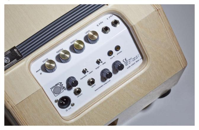
• two guitar input jacks, normal (A) and low gain (B)
